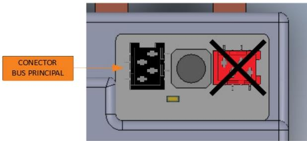
Figura 10 Detalle conector negro del bus principal
