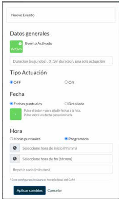
Figure 29 Scada web – ON/OFF event
