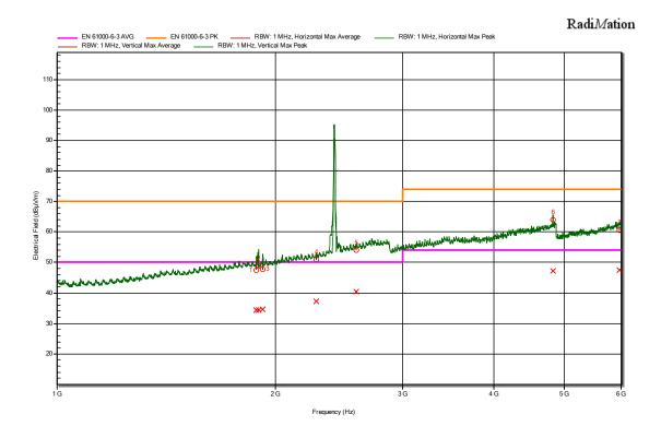
NOTE: The frequency band from 2.280 MHz to 2.607,675 MHz is excluded from radiated emission measurements, as per ETSI EN 301489-17 v2.2.1.
